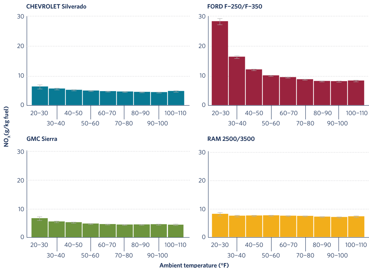
Figure 8. Average NO x emissions by ambient temperature for each vehicle model. Error bars represent the 95% confidence interval.
