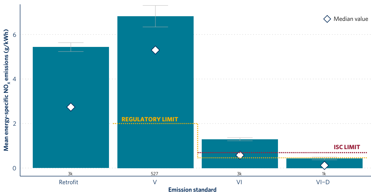
Figure 19. Mean and median energy-specific NO x emissions (g/kWh) of buses measured during the 2022 emission testing in Scotland by emission standard and retrofit status. Whiskers represent 95% confidence interval of the mean and diamond shape indicates the median NO x emissions (g/kWh). Only measurements of over 100 are presented.
