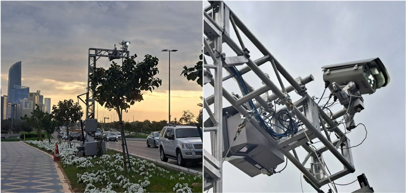
Figure 1. HEAT EDAR remote sensing device measuring emissions from passing vehicles in Abu Dhabi. Source: Oriol Teixidó, former project lead at EAD.
