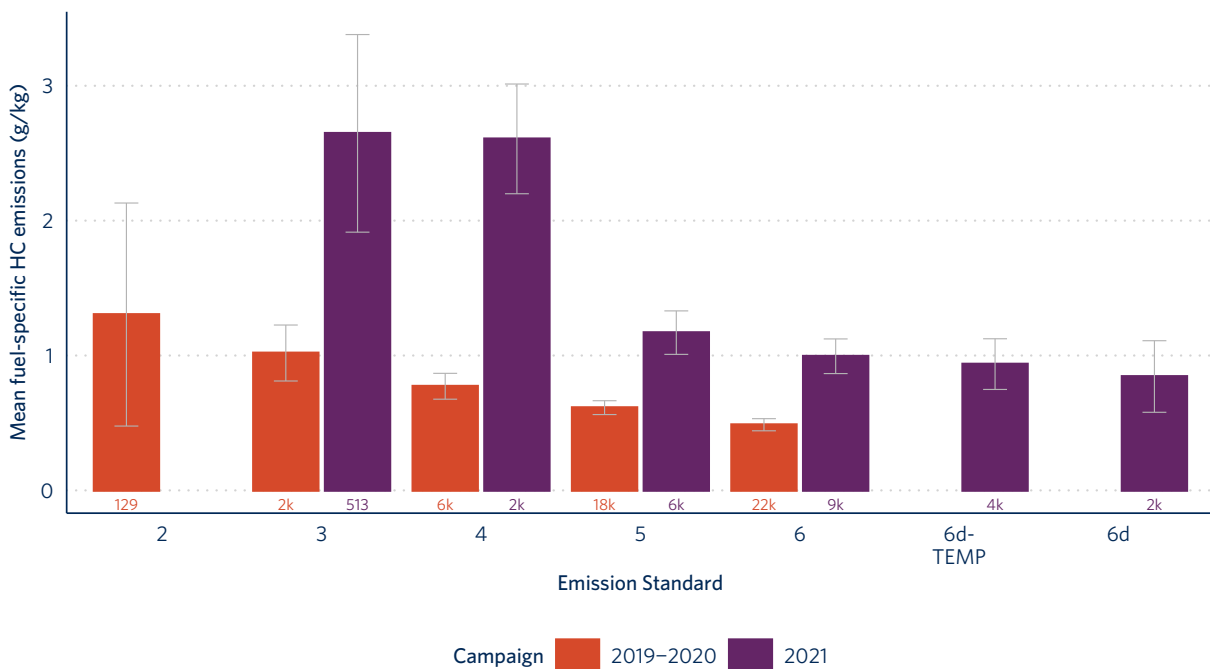
Figure 33. Mean fuel-specific HC emissions from light-commercial vehicles by Euro standard measured in 2019-2020 and 2021. HC emission measurements were not available for the 2017 measurements. The number of measurements is presented below each bar and only measurements of over 100 are presented. Whiskers represent 95% confidence interval to the mean.
