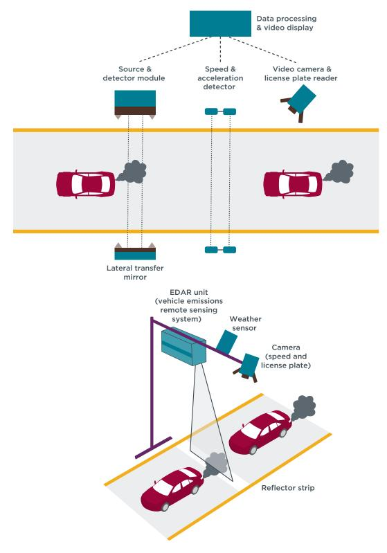
**Figure 1.** Schematic setup of the three units of the remote sensing device. Top, setup for cross-road remote sensing: the light source with the reflecting mirror at the other side of the road and the light detector; the speed and acceleration detectors; and the number plate recorder. Bottom, setup for top-down remote sensing system (EDAR).
