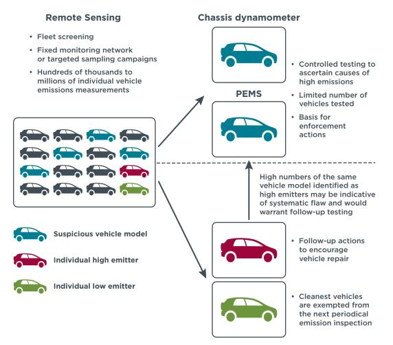
**Figure 2.** Conceptual diagram showing possible applications of vehicle remote sensing in an enhanced vehicle emission control program.
