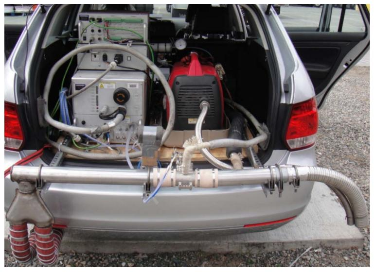
Besch et al., WVU 2014 – PEMS testing leading to dieselgate revelation
