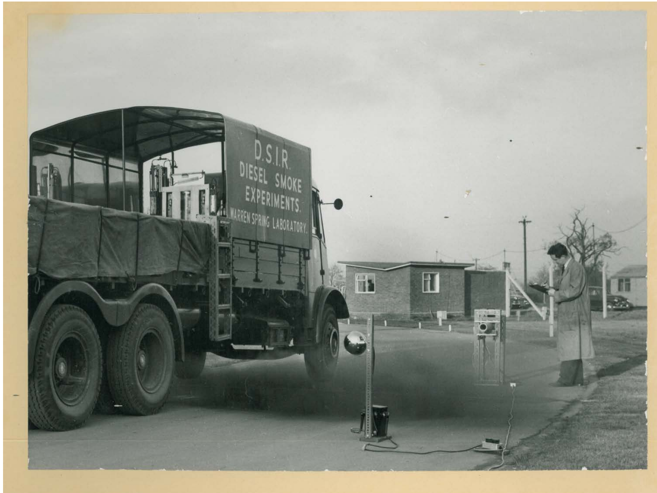
Early 'remote sensing' measurements at the Warren Spring Laboratory (predecessor to Ricardo Energy & Environment) from the early 1960s
